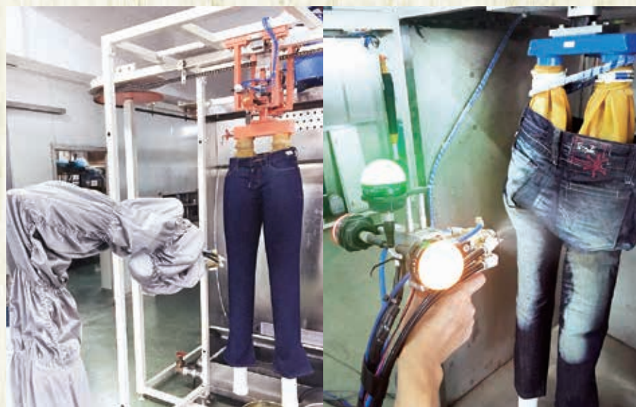
系統設有六軸機械手和可編程噴槍，可快速學習噴塗技術員的動作。With the six-axis manipulator and the programmable spraying gun, the system can learn the trajectory motions of manual operators.
